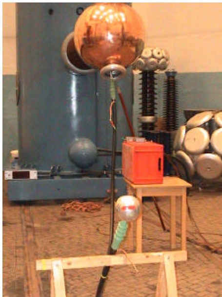
Figure 1: a) Diagram of the test setup. b) Photo of the test setup. c) Detailed Photo of the needle placed on a sphere (grinded tungsten needle with a diameter of 0.8 mm from tungsten inert-gas welding).
