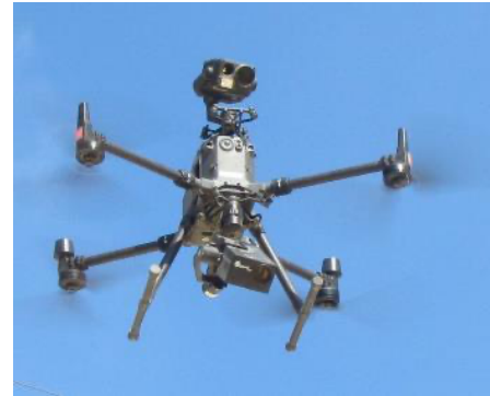
Simultaneous UV and IR Inspection on DJI M300
