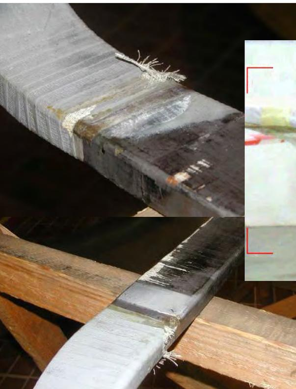
Left: visual inspection; Right: UV inspection, PD on the interface between semi-conducting and gradient coating
