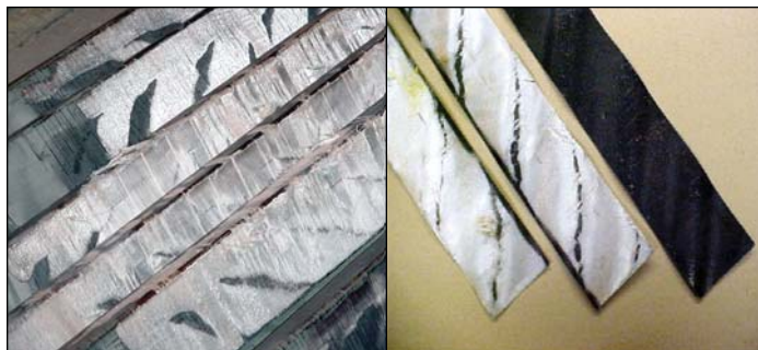
Ladder effect due to loose stator windings (above, left). The effects of mechanical and corona damage to side ripple springs (above, right).
